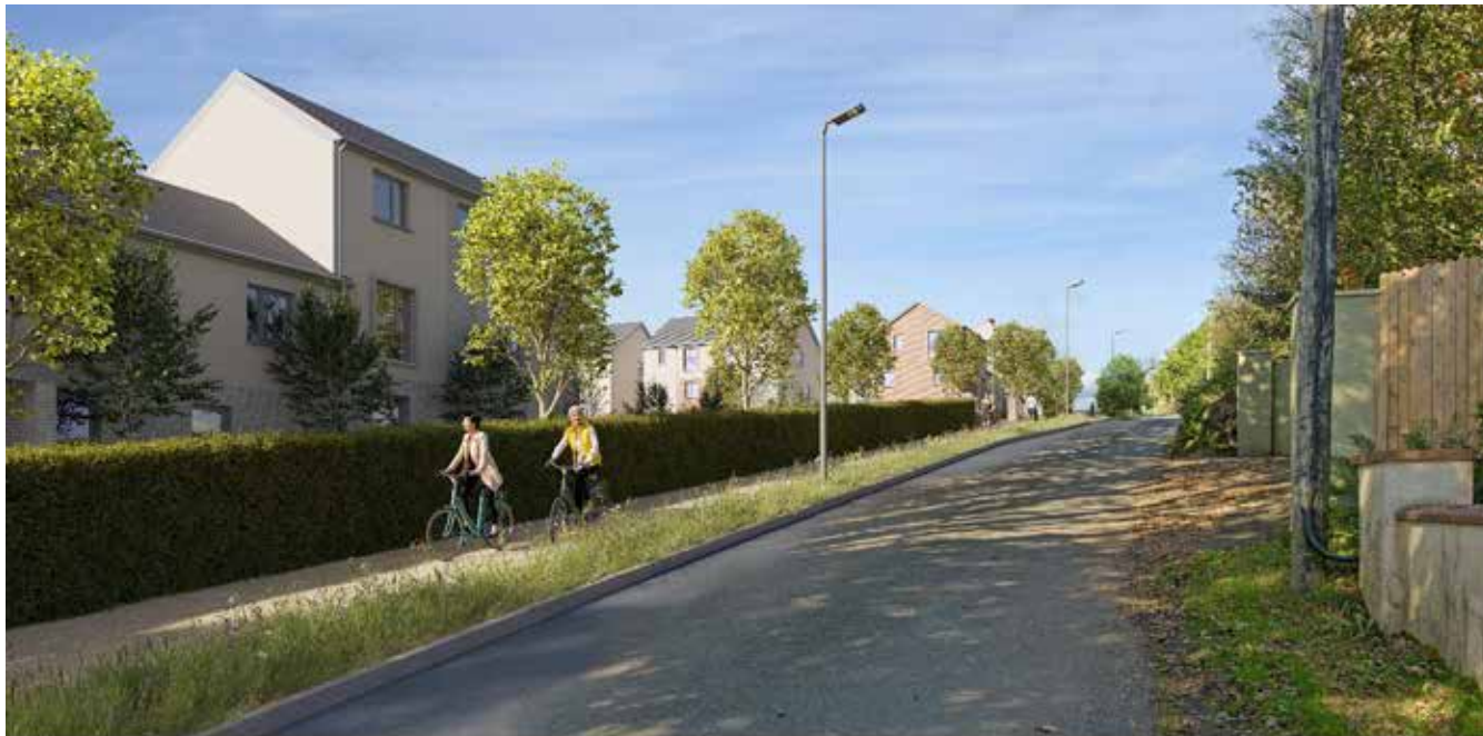
Figure 5-4 Proposed treatment of the Kilnahue Lane road corridor, including (a) removal of the existing roadside hedgerow and trees, (b) widening of the road surface for safe two-way traffic, (c) provision of a segregated pedestrian and cycle path, and (d) a wide green corridor comprised of a hedge, grass verge and trees to maintain the road's green/leafy character.
